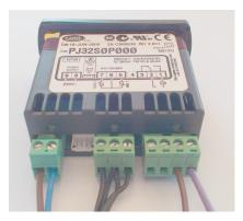
Having removed the PG32 from the fascia of the refrigerator, you will see three connector blocks at the rear of the controller. These are a 2 pin (power in), a 3 pin (sensors) and a 4 pin (compressor out, only two pins used).
